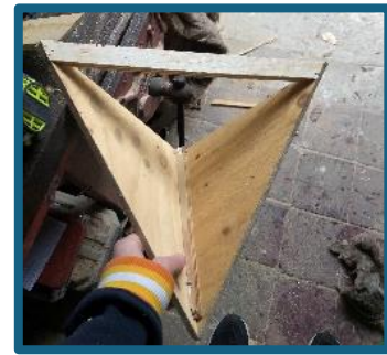
Building the bass traps using ply
